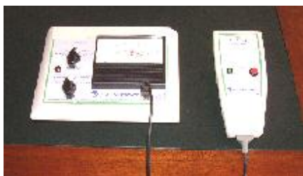
Fig. 1 Infrared Desktop Diagnostic Scanner: Meter console (left) and hand-held scanner (right). The meter console is equipped with 'sensitivity' and 'function' control knobs.
